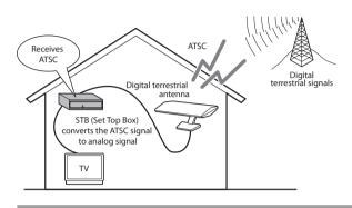
This STB makes it possible to view the digital TV programs on your analog TV by converting the digital signal to the analog signal. You can use most features provided by the digital broadcast, except that the resolution of the image is always output in 480i (standard resolution).
