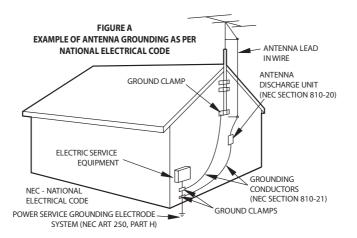
conductors, location of antenna-discharge unit, connection to grounding electrodes, and requirements for the grounding electrode. (Fig. A)
