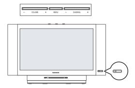
Should your remote control be lost or broken you can still change some of the basic settings with the buttons on the top of your TV. Press the power switch  $\phi$  to switch the TV on. Press:
