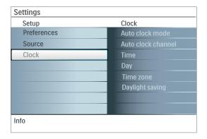
Most TV channels do not transmit clock information. A few cable channels do, but they are at the end of the channel ring. Antenna channels do not transmit clock information. If clock information does not appear, you can assume that either clock extraction is taking a long time or that there is no clock.
