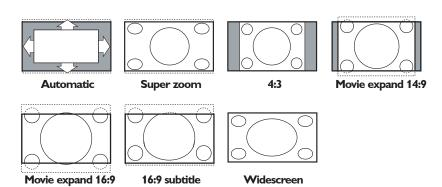
Automatic makes the picture fill the screen as much as possible. It is recommended to press the cursor up/down or left/right key to adjust the picture position on the screen.
