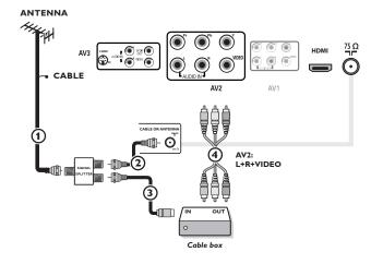
Note: Video In signal input can be handled by AV2, AV3 as well.
