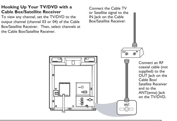
Your Cable Box/Satellite Receiver may have Audio and Video Out jacks instead of the single Antenna Out jack (RF coaxial or 75 ohm) shown here. If so, connect Audio and Video cables to the Audio/Video Out jacks of the Cable Box/Satellite Receiver and to the AUDIO/VIDEO In jacks on the front of the TV/DVD. Press SELECT on the remote to set the TV/DVD to AUX, not channel 3 or 4. Select channels you want to watch at the Cable Box/Satellite Receiver as usual, leaving the TV/DVD on AUX.
