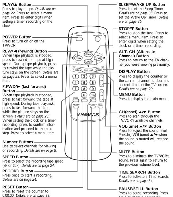
Press to pause recording. Press again to resume recording. Details are on page 24. During tape playback, press to freeze the picture (still). Details are on page 23.
