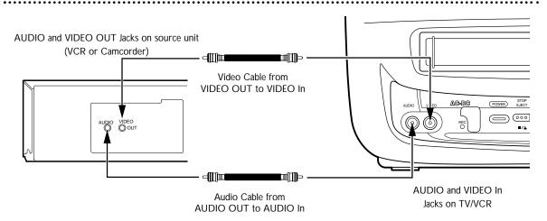
Make the connections shown above, using audio and video cables (not supplied). Connect the source unit (VCR or camcorder) to a power source after connections are made.
