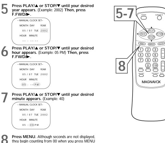
**Press MENU.** Although seconds are not displayed, they begin counting from 00 when you press MENU on the remote control. Use this feature to synchronize the clock with the correct time.
