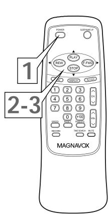
Press PLAY/▲ or STOP/▼ to select AUTO PRESET. Then press F.FWD/►. The TV/VCR scans and memorizes all active channels in your area. When scanning is complete, the TV/VCR will go to the lowest available channel automatically. Use the CH(annel) ▲/▼ buttons to select memorized channels. Use the Number buttons to select non-memorized channels.
