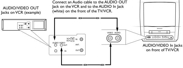
Connect a Video cable to the VIDEO OUT Jack on the VCR and to the VIDEO In Jack (yellow) on the front of the TV/VCR.
