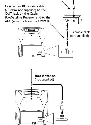
Hooking Up Your TV/VCR With a Cable Box/Satellite Receiver To view any channel, set the TV/VCR to the Cable
