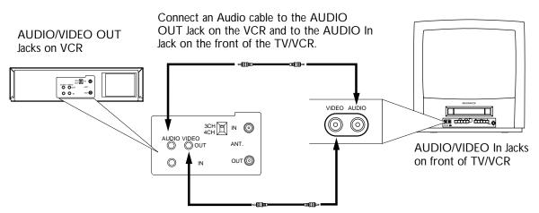
Connect a Video cable to the VIDEO OUT Jack on the VCR and to the VIDEO In Jack on the front of the TV/VCR.
