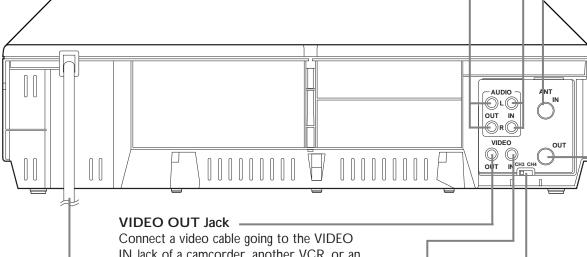
IN Jack of a camcorder, another VCR, or an audio-visual system (monitor, laser disc player, digital video disc player, etc.) here. Details are on pages 34 and 40.
