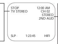
The indication 2ND AUD or STEREO that appears on this side of the status display tells you if the program you're watching is available in second audio or stereo. This indication is not available during tape playback.
