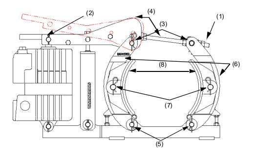
**9.1.(a).(xii):** Before starting shoe installation, check that the brake surface of the wheel is clean and free from oil and grease.
