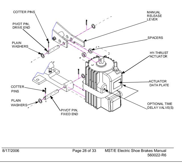
**9.2.(f):** Secure or support the actuator before attempting to remove the pivot pins.
