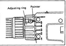
Before actual operation, drive a trial screw into your material or a piece of duplicate material to determine which torque level is required for a particular application.
