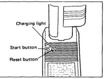
goes out within 10 seconds even after pressing the reset button and start button a couple of times, the battery cartridge is dead. (CAUTION: Wait for more than 5 seconds after the charging light goes out to press the reset button again.) Replace it with a new one. When the charging light goes out after about one hour, you may remove the fully charged battery cartridge.
