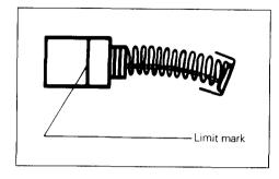
Use a screwdriver to remove the brush holder caps. Take out the worn carbon brushes, insert the new ones and secure the brush holder caps.
