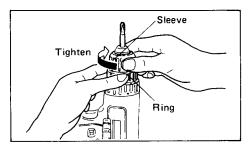
To remove the bit, push the sleeve up toward the "FREE" side and turn the sleeve counterclockwise while holding the ring with your other hand.
