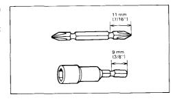
To install the bit, pull the sleeve in the direction of the arrow and insert the bit into the sleeve as far as it will go. Then release the sleeve to secure the bit.
