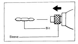
To remove the bit, pull the sleeve in the direction of the arrow and pull the bit out firmly.
