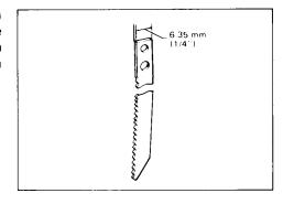
Insert the blade into the blade holder as far as it will go. Make sure that the end of the blade shank reaches the bottom of the inner slit and tighten the bolt securely with the hex wrench.
