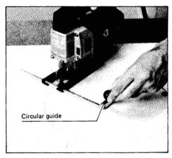
To attach the circular guide, use the pin, inserting it in the center hole (arrow) and secure it with the threaded knob. Then slide the base of the tool forwards. The circular guide attaches to the base of the tool in the same manner as the guide rule (rip fence).
