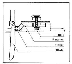
Use a lubricant or cutting oil between the blade and roller when cutting metals. Failure to do so will shorten the service life of your blade and roller.
