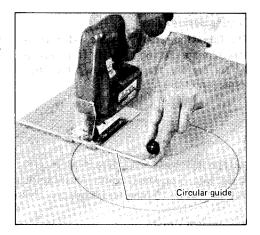
When attaching the circular guide, use the pin, inserting it in the center hole (arrow) and secure it with the threaded knob. The circular guide attaches to the base of the tool in the same manner as the guide rule (rip fence).
