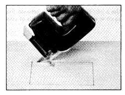
If using a drill for a starting hole, bore a hole over 12 mm (1/2") in diameter. Then insert the blade in it and proceed.
