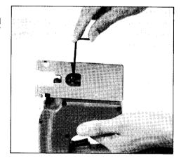
Loosen the bolt on the back of the base with the hex wrench. Tilt the base to the desired angle. The edge of the housing indicates the bevel angle.
