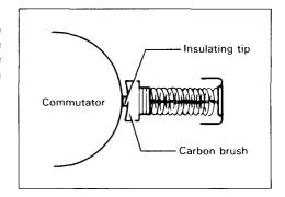
Use a screwdriver to remove the brush holder caps. Take out the worn carbon brushes, insert the new ones and secure the brush holder caps.
