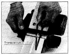
while lightly holding the triangular rule flush against the rear base. The triangular rule flush against the rear base. The triangular rule will be lifted very slightly and will be moved forward (toward the front base). The triangular rule should move forward 1-5 mm (3/64''. 13/64''). Check the blade protrusion at both ends of the blade. The triangular rule should move forward equally at both ends. If the blade does not protrude properly, use the blade gauge to adjust the blade protrusion.
