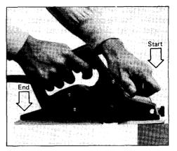
rough cutting, the depth of cut can be increased, while for a good finish you should reduce the depth of cut and advance the tool more slowly.
