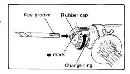
Turn the change ring in the direction of the arrow until the mark on the change ring is aligned with the mark on the rubber cap to secure the bit.
