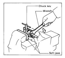
Remove the screw from the chuck adapter assembly and screw the chuck adapter into the drill chuck. Use a wrench to tighten the chuck adapter securely, applying about  $300-400 \text{ kgf} \cdot \text{cm}$  ( $21.6-28.9 \text{ lb} \cdot \text{ft}$ ) torque. [Note: you can obtain  $300-400 \text{ kgf} \cdot \text{cm}$  ( $21.6-28.9 \text{ lb} \cdot \text{ft}$ ) torque by applying pressure of 30-40 kg (66-88 lbs) to the wrench while holding the portion 10 cm (4") from the wrench head.]
