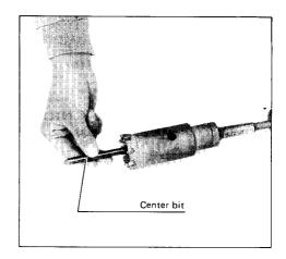
Rest the core bit on the concrete and turn the tool on. Once the core bit has cut a shallow groove into the concrete, remove the center bit. Then resume drilling.
