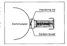
Use a screwdriver to remove the brush holder caps. Take out the worn carbon brushes, insert the new ones and secure the brush holder caps.
