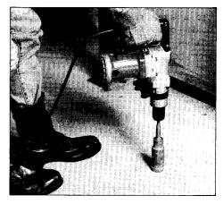
To remove the core bit, hold the adapter with the wrench, insert the rod into the hole in the core bit and tap with a hammer to unscrew.
