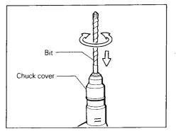
If the bit cannot be pushed in, remove the bit. Pull the chuck cover down a couple of times. Then insert the bit again. Turn the bit and push it in until it engages.
