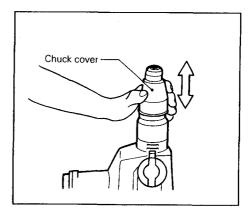
After installing, always make sure that the bit is securely held in place by trying to pull it out. To remove the bit, pull the chuck cover down all the way and pull the bit out.
