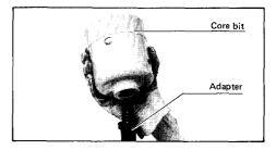
Rotate the change lever to the  $\widehat{\square}$  position. Rest the core bit on the concrete and turn the tool on. Once the core bit has cut a shallow groove into the concrete, rotate the change lever to the  $\widehat{\square}$  geposition and resume drilling.
