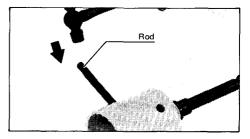
[When not using the center bit] Screw the core bit on the adapter. Install the adapter with the core bit in the tool in the same manner as a drill bit.
