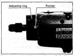
Before actual operation, drive a trial screw into your material or a piece of duplicate material to determine which torque level is required for a particular application.
