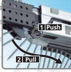
Screw strip also can be removed in the direction of the arrow by pushing
