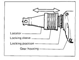
Initially, adjust the locator assembly to create a distance of approximately 1 mm (3/64") from the tip of the locator to the base of the screw head. One full turn of the locator equals 1.5 mm (1/16") change in depth. After adjusting the locator assembly, push the locking sleeve in to lock the locator in place. Drive a trial screw into your material or a piece of duplicate material. If the depth is not suitable for the screw, continue adjusting until the proper depth setting is obtained.
