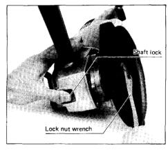
To remove the wheel, follow the installation procedure in reverse.
