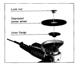
To tighten the lock nut, press the shaft lock firmly so that the spindle cannot revolve, then use the lock nut wrench and securely tighten clockwise.
