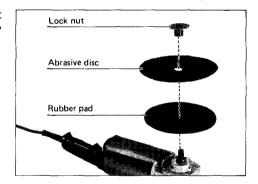
To tighten the lock nut, press the shaft lock firmly so that the spindle cannot revolve, then use the lock nut wrench and securely tighten clockwise.
