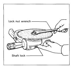
To remove the disc, follow the installation procedure in reverse.
