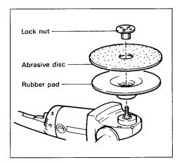
To tighten the lock nut, press the shaft lock firmly so that the spindle cannot revolve, then use the lock nut wrench and securely tighten clockwise.
