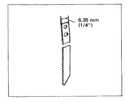
Insert the blade into the blade holder as far as it will go. Make sure that the end of the blade shank reaches the bottom of the inner slit and tighten the bolt securely with the hex wrench.
