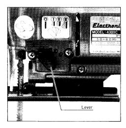
Position 0 — For cutting in mild steel, stainless steel and plastics.
