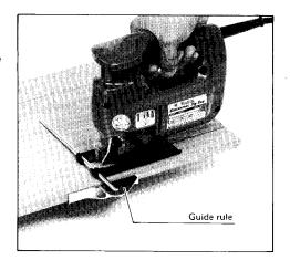
To attach the guide rule (rip fence), secure the rule holder to the base with the screw (do not tighten).
