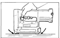
If the staples are driven too shallow, press the tool head as shown in the figure and drive the staples.
