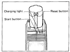
the start button (red). If the charging light goes out within 10 seconds even after pressing the reset button and start button a couple of times, the battery cartridge is dead. (CAUTION: Wait for more than 5 seconds after the charging light goes out to press the reset button again.) Replace it with a new one. When the charging light goes out after about one hour, you may remove the fully charged battery cartridge.
