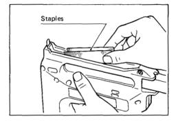
To secure the sub-magazine in place, push the sub-magazine while pressing the plate spring on the rear of the sub-magazine.
