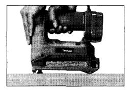
If the tool becomes jammed, do as follows. First, remove the battery cartridge. Open the sub-magazine and remove the stuck staple using a screwdriver or the like.
