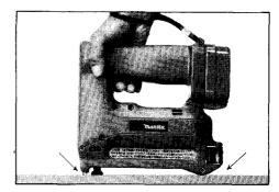
If the staples are driven too shallow, press the tool head as shown in the figure and drive the staples.
