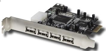
Thank you for purchasing the MANHATTAN® Hi-Speed USB 2.0 PCI Express Card, Model 160391. Compliant with PCI Express 1.0a and Hi-Speed USB 2.0 specifications, this card fits PCI Express x1, x2, x4, x8 and x16 lane buses and adds five Hi-Speed USB 2.0 ports (four external and one internal) to desktop computers, with each port able to support data transfer rates of up to 480 Mbps.
