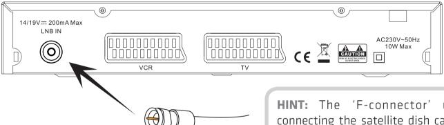
Connect the cable from your dish to the LNB IN socket at the back of the receiver (if the dish cable is fitted with a wall socket inside your home, you will need a connecting cable, which you can get from your installer).
