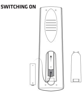
Take the battery compartment cover off the back of the Plaza DS•100 remote control by lifting it up while pushing the catch. Insert the two AAA batteries supplied, as shown on the inside of the compartment, and replace the compartment cover.
