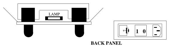
**D- FUSE COVER-** Pry in the small slot to move the locking tab towards the fuse cover and it should pop open. Only use an MDL 3 fuse if it needs replacing (MDL 2 for 220V units).
