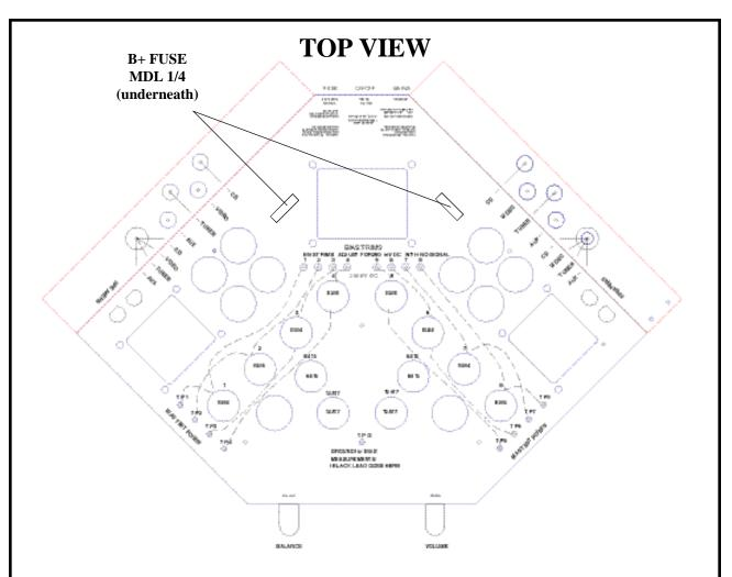
**TUBE LOCATIONS** - See the diagram above for the proper tube locations. Power should be unplugged and the tubes cool before handling them. We label the tube sockets, test points and trimmers to help. It is possible to put tubes in wrong if you bend the pins - not good. On this diagram we added dashed lines to further clarify which test points are associated with which tube and which trimmer but they are numbered right on the chassis.
