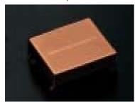
requirements of Marantz. Marantz developed it's own discrete circuit boards to replace the IC's. These HDAM's consists of discrete surface mount components with short mirror image L/R signal paths. These devices are
