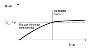
Conversely, you should be aware that if the sync level setting is too low, the noise level of an analog source may be higher than the sync level, so that sync recording fails to start.
