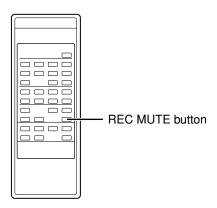
The display will indicate "Rec Mute" and muted recording will begin. After approximately four seconds, the recorder will enter record-ready mode.
