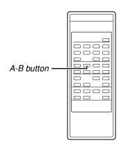
1 During playback, press the A-B button on the remote control unit at the point (A) where you want to start A-B repeat playback.
