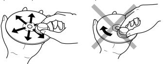
Wipe in a radial direction. Do not wip
