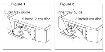
• Place 3 inch/8 cm discs in the inner tray guide without using an adapter.
