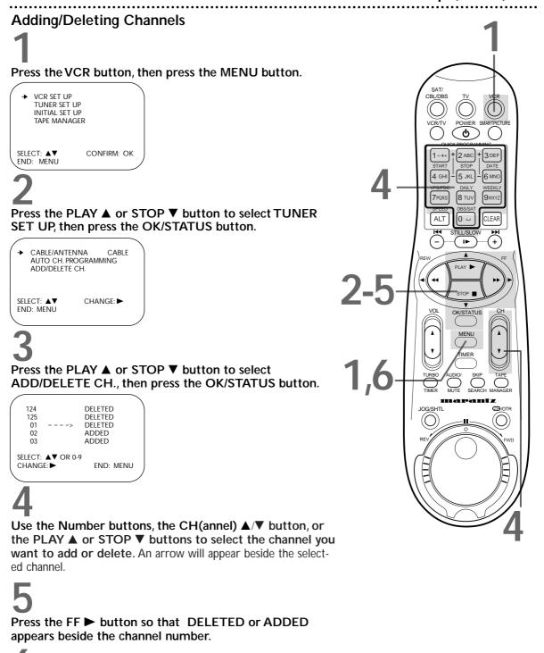
**Press the MENU button.** Programming of the last channel you added or deleted will appear on the screen.
