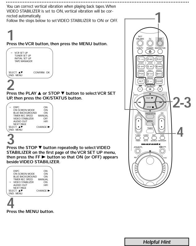
Regardless of the setting, this feature has no effect during recording or special effects playback.
