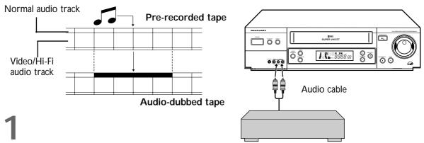
Connect an audio component to your VCR's AUDIO IN L+R connectors. When connecting monaural equipment, use only the VCR's AUDIO IN L connector.
