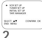
Press the PLAY  $\blacktriangle$  or STOP  $\checkmark$  button to select INITIAL SET UP, then press the OK/STATUS button.
