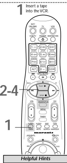
The Program Overlap Warning does not function with Turbo Timer. The timer recording with the earliest start time will record. Then, the remaining portion of the later recording will record.
