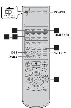
You can directly program the VCR's timer to record up to 24 broadcasts, as far as a year in advance. Remember, the clock must be set before you can program the timer ( pg. 10).
