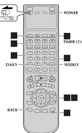
Timer recording allows you to program the VCR to automatically record a broadcast at some future time. Up to 24 timer recording programs can be made using VCR Plus+ timer programing or Express timer programing method ( pg. 38) as far as a year in advance.
