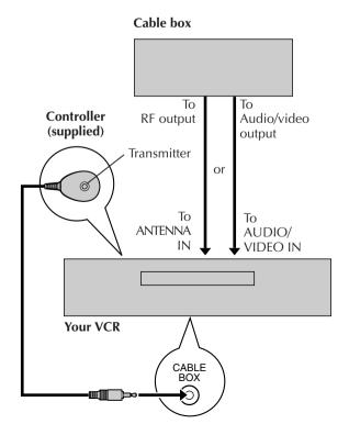
The following procedure is required if you receive your TV channels through a cable box (descrambler). The Controller allows the VCR to automatically switch the cable box channel during timer recording. The Controller is effective for recording broadcasts that have been programed using VCR Plus+ (F) pg. 34) or Express timer programing (F) pg. 38).
