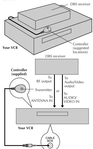
The following procedure is required if you receive satellite channels through a DBS (Direct Broadcast Satellite) receiver. The Controller allows the VCR to automatically switch the DBS receiver's channels during timer recording.
