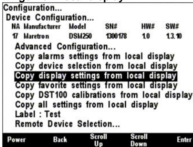
Figure 68 – DSM150/DSM250 Copy display settings from local display
