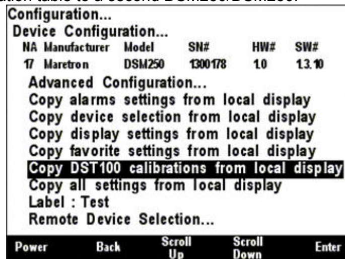
Figure 71 – DSM150/DSM250 Copy DST100 calibrations from local display
