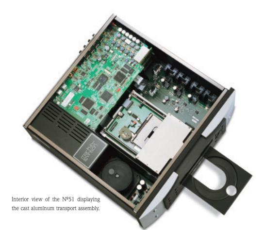
it from the audio section and other sections of the player. The damper bridge is machined from solid aluminum, increasing mass and rigidity, thus helping to eliminate flexure from day-to-day operation and promoting stability in the physical mechanism. All of these design attributes work in concert to provide smooth, quiet, and consistent transport operation.
