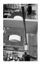
11. Carefully lift connector ends of cables out of holes in phono preamp top cover.
