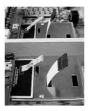
12. Plug all four cables from phono preamp modules into their respective sockets on upper circuit board inside N°32 Preamplifier.
