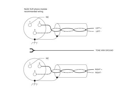
Combined with a shielded, twisted pair cable from cartridge to preamp, the XLR input phono preamp offers the ultimate in noise rejection and low level signal resolution. (An RCA-equipped version is also available for wider compatibility with existing phono cables.)
