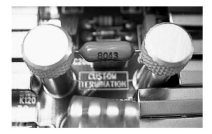
8. Trim lead if necessary to avoid contact with other components.
