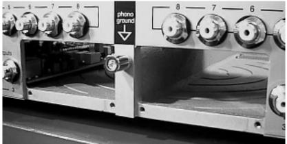
7. Make sure cables on top of phono preamp modules have connector ends in holes in top cover. The ribbon cables on the top of the phono modules should have
