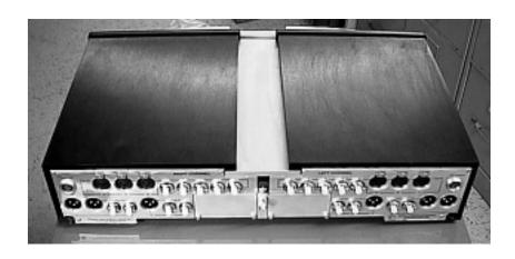
3. Remove the two screws from rear bottom of N°32 Preamplifier top cover that hold it in place (using the <sup>3</sup>/<sub>32</sub>" hex key supplied with the N°32).
