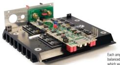
Each amplifier channel utilizes two current-gain (CG) boards for the balanced output drivers. The CG boards are made from Arlon 25N, which was chosen for its superior dielectric characteristics. Simply the Finest Home Audio and Video Components Built Today.
