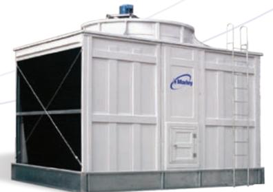
**Marley NC<sup>®</sup> Fiberglass Cooling Tower**—Fiberglass, field-erected, crossflow cooling tower designed to serve air conditioning and refrigeration systems as well as light or medium industrial process loads on clean water. Structure is available in galvanized or stainless steel. Cells available from 105 to 942 tons per cell. CTI Certified. Not available in the US, Canada or Europe.
