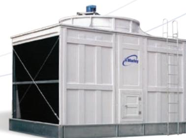
**Marley NC® Fiberglass Cooling Tower**—Fiberglass, field-erected, crossflow cooling tower designed to serve air conditioning and refrigeration systems as well as light or medium industrial process loads on clean water. Structure is available available in galvanized or stainless steel. Cells available from 105 to 942 tons per cell. CTI Certified. Not available in the US, Canada or Europe.
