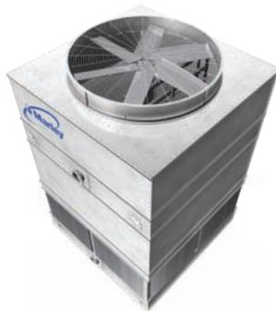
**Marley MD Cooling Tower**—Counterflow, induced-draft design requires less plan area than crossflow towers. Factory assembly is standard and the MD is available in galvanized or stainless steel. Tower available from 165 to 500 tons per cell. Five-year mechanical equipment warranty. CTI Certified.
