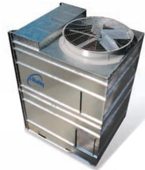
**Marley AV Cooling Tower**—Singleflow, induced-draft crossflow design offers pump and fan energy savings in a small footprint installation. Factory assembly is standard and the AV is available in galvanized or stainless steel. Tower cells available from 117 to 390 tons per cell. CTI Certified.
