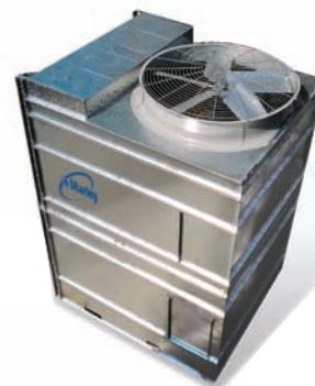
**Marley AV Cooling Tower**—Singleflow, induced-draft crossflow design offers pump and fan energy savings in a small footprint installation. Factory assembly is standard and the AV is available in galvanized or stainless steel. Tower cells available from 117 to 390 tons per cell. CTI Certified.
