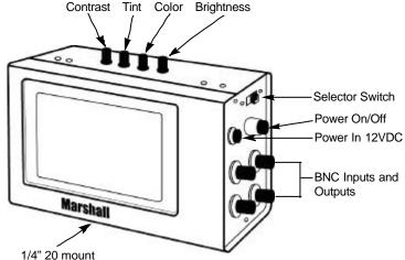
when power is supplied to the monitor. The monitor also has a 1/4-20 mount located on the bottom of the unit. This is useful when mounting the monitor on the top of a camera by using a hot shoe mount (Marshall part# V-LCD-MT) or other mounting devices.
