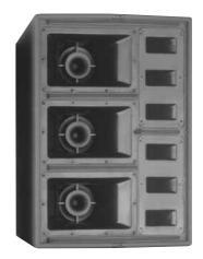
The W8CT utilises a total of 6 x I" (25mm) exit high frequency drivers, optimised for maximum efficiency in the band from 3.5kHz upwards. The I" (25mm) exit drivers used are extremely efficient in this band and can produce enormous high frequency energy by virtue of their vertical line array configuration. Use of I" (25mm) exit drivers is additionally important as it means that the HF array elements can be more closely spaced.
