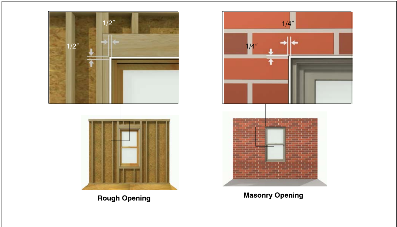
Figure 2: Preparing openings for concrete block openings.
