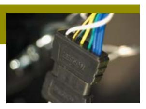
ball does not have to act as an electrical connection. Always have your light plug hooked up when backing your trailer. Disc brakes will not release without the special connector wired to your back-up lights on your tow vehicle.
