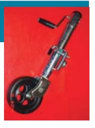
Like any mechanical assembly, a jack requires maintenance to function properly over a long period of time. The drive gear and the rack-and-pinion should be greased. The caster and wheel bearing should be oiled frequently. Failure to swing up the jack before towing may result in damage to your trailer.
