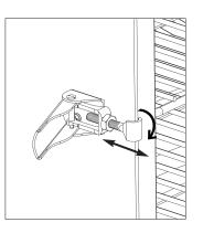
Loosen hex nut on door latch. Turn hook clockwise to tighten as shown. Secure hex nut firmly against door latch.
