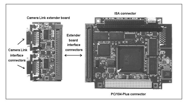
Three of these connectors are located on the main board, and three are located on the extender board.
