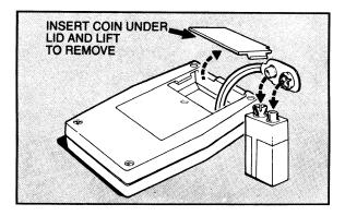
Turn Ski Slalom game over, face down. Remove battery door. Attach one 9-volt alkaline transistor battery to connector. Replace battery door.
